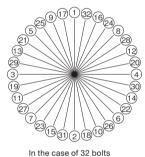
able 13) Bolt Tightening Torque for Mounting Model RW
