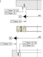
Machining accuracy of peripheral part
