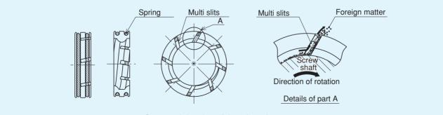
Structural drawing of the wiper ring
